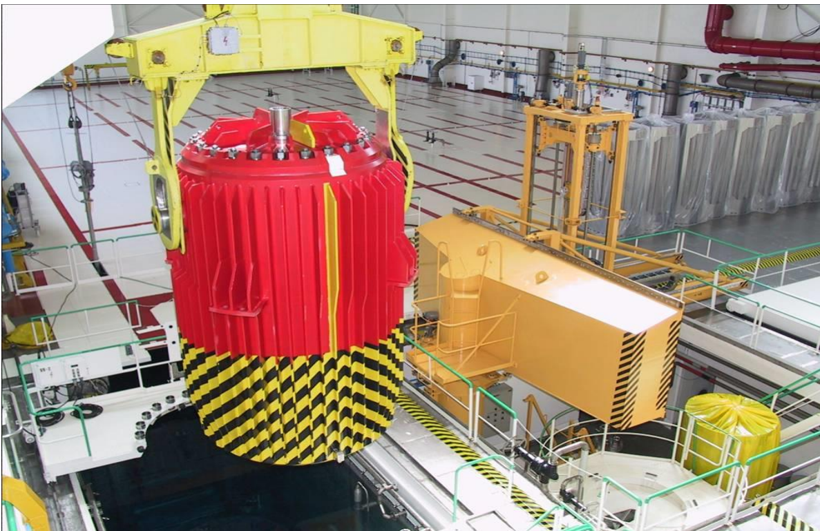
Fig. 14: Transport of TK C-30 by special transport hitch
