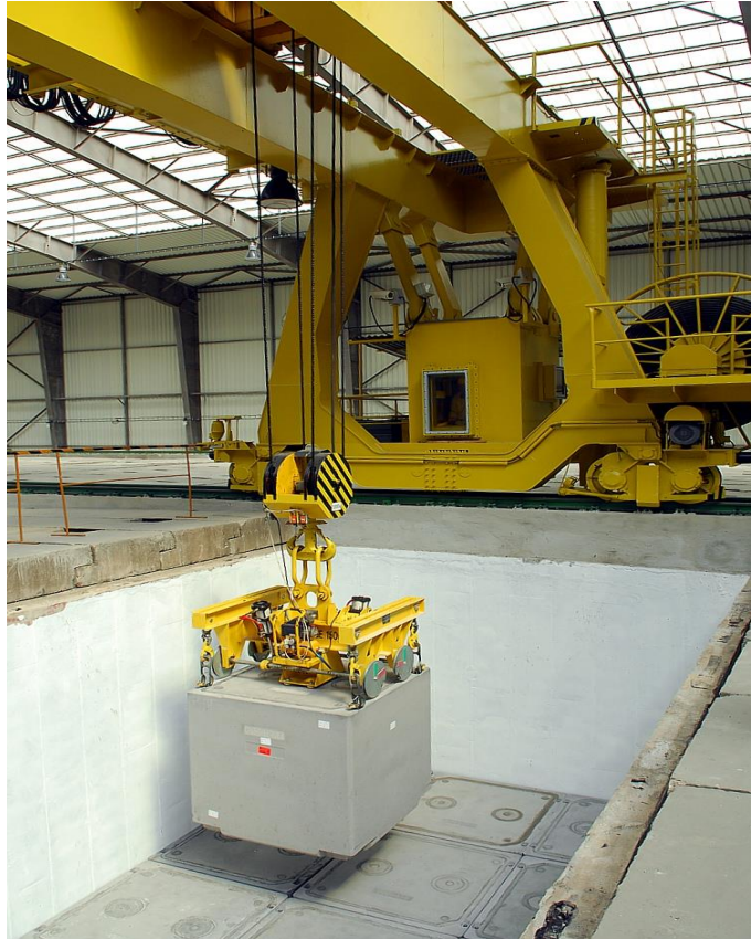
Fig. 21: VKB after measurements taken at Gamma scanner prior to disposal into disposal boxes of the repository arranged as double-rows
