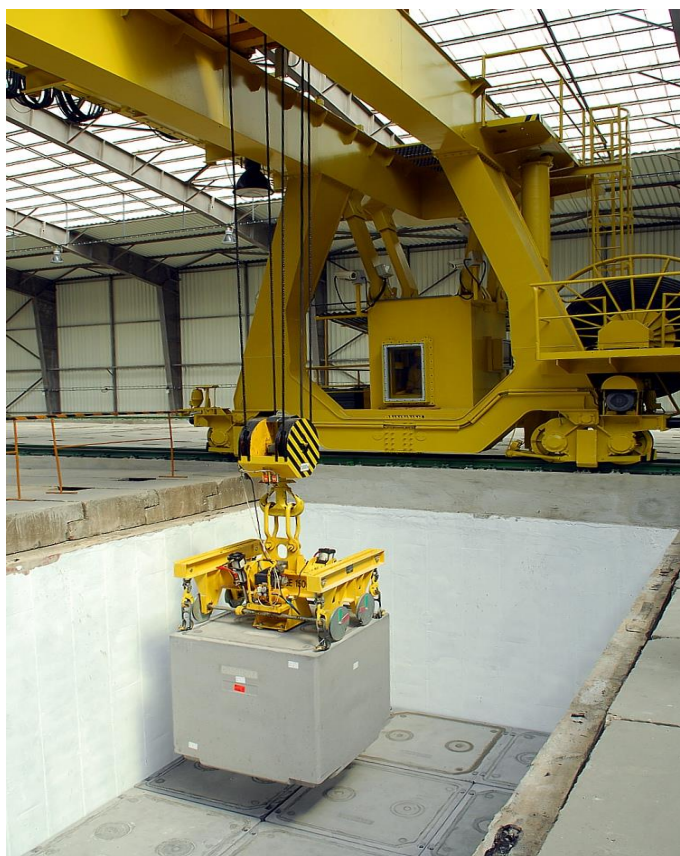
Fig. VBK after measurements taken at Gamma scanner prior to disposal into disposal boxes of the repository arranged as double-rows
