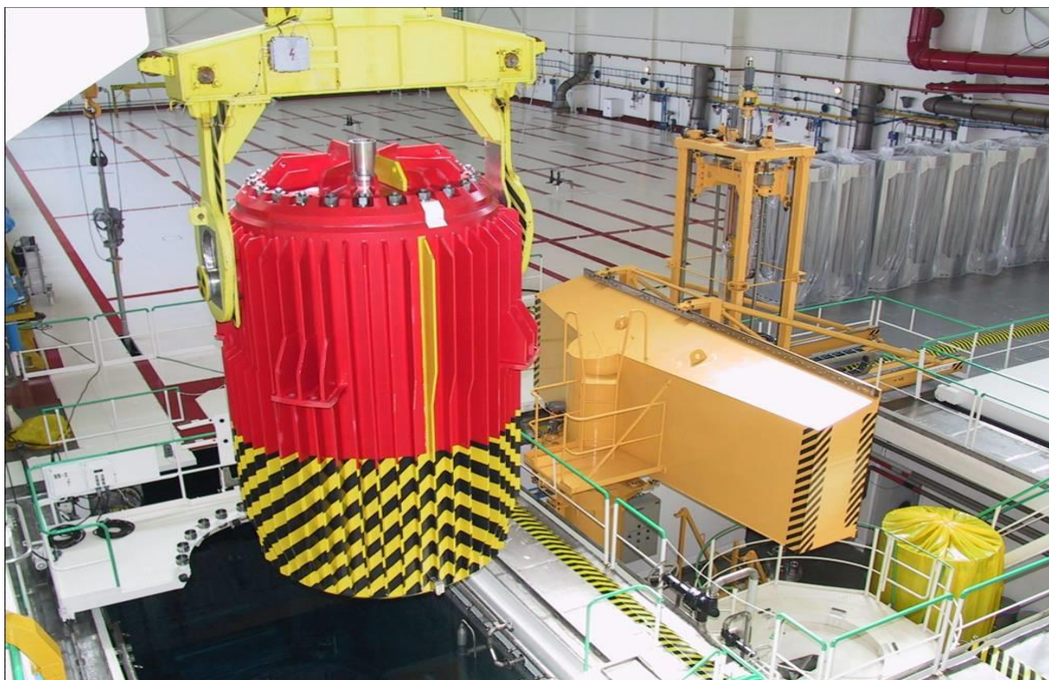
Fig. Transport of TK C-30 by special transport hitch
