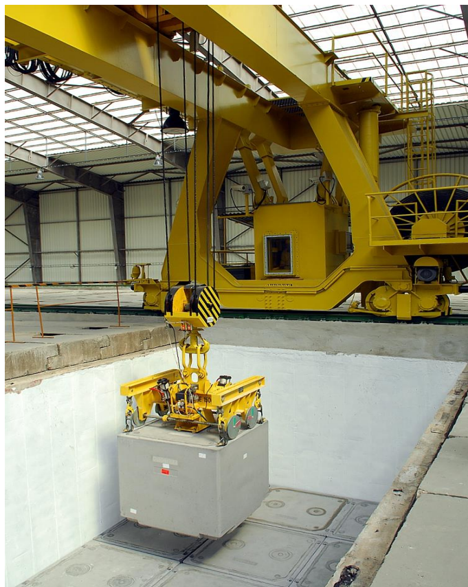
Fig. 19: VBK after measurements taken at Gamma scanner prior to disposal into disposal boxes of the repository arranged as double-rows
