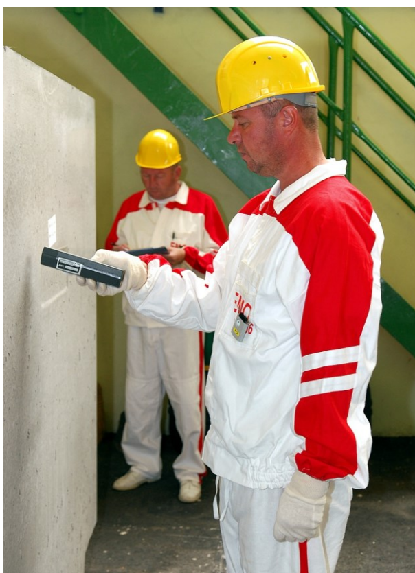
Fig. F.4.2 Monitoring of radioactivity on the surface of fibre-concrete containers
