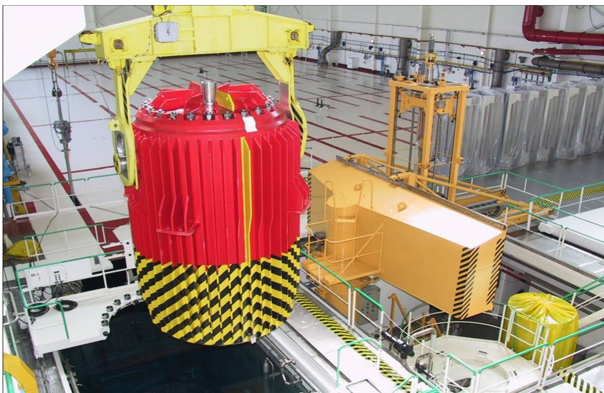
Fig. D.1.2d) Transport of TK C-30 by special transport hitch
