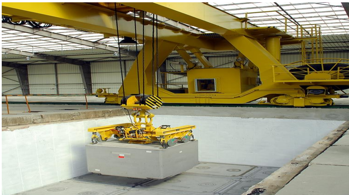
Fig. D.2.6 Disposal of VBK to disposal boxes of the repository in the first double row
