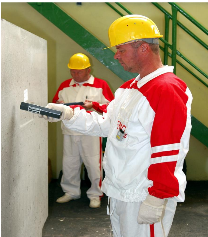
Fig. Monitoring of radioactivity on the surface of fibre-concrete containers
