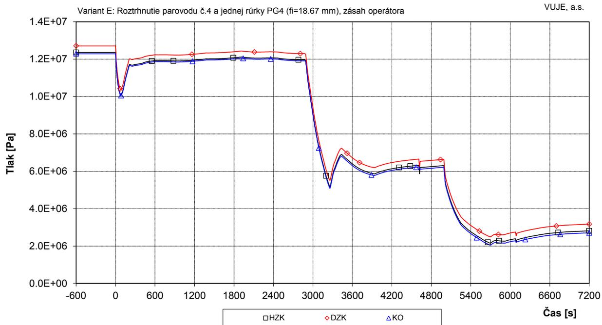
Obr. 7.2.1.15.11-E-1: Tlak v I.O.
